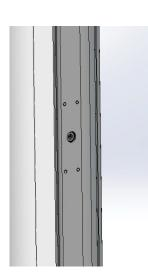
Insert the t-handle and turn counterclockwise to open the front door.
