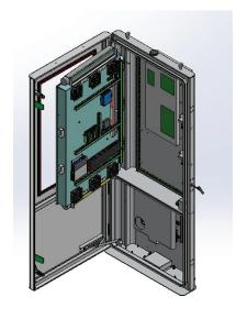
Route antenna wires down thru the cable ducting in the rear of the chassis and then across and up into the rear of the monitor pan and into cradle. Remove the lower power cover panel located in the bottom center of the chassis.
