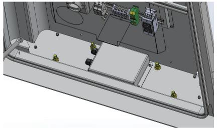
Once the front door is open, remove the four bolts holding this down to the pallet.
