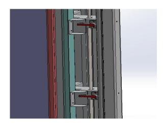
Locate the red handled clamps o the right side and turn counterclockwise to allow rear monitor pan to swing out.
